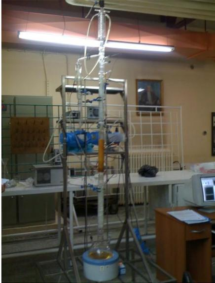
Fig.1. Reactive packed distillation pilot plant
