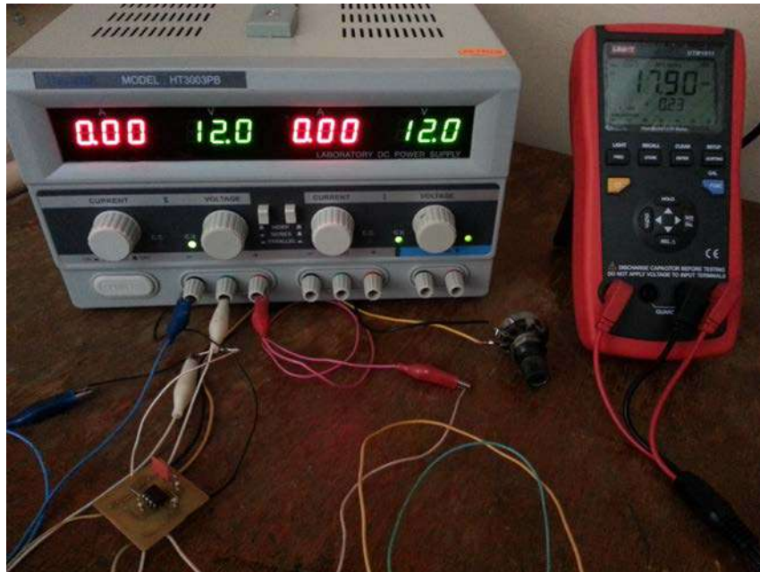
Fig. 4. Practical realization of the equivalent of inductance ( L = 17.9 \text{ mH} )
