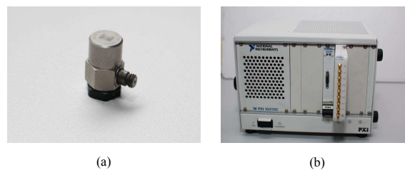
Fig. 1. The data acquisition setup: (a) accelerometer, (b) PXI system.
